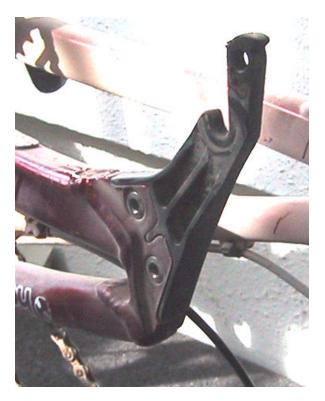
First remove the rear wheel and rear derailleur. Using a 5mm allen and a chainring nut wrench remove the two chainring bolts. Using a 2.5mm Allen loosen the two small setscrews a few turns. You may need to tap the drop out with the soft blow hammer to get it off the frame.
